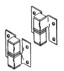
About the product: Stamped stainless steel square barrel surface mounted hinges have hole centers of 1-1/2" vertically and 2-7/16" horizontally. The overall size is 3-1/8" wide x 3" high. Comes complete with one pair of hinges and all attaching hardware to hang one door.
